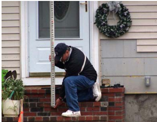
(Kennebunk, ME) Field staff measures flood levels after 2007 nor-easter.
