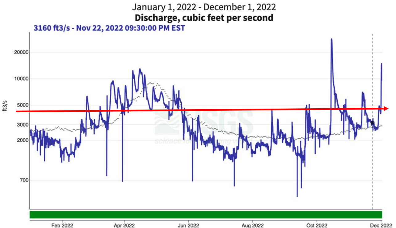
Figure 1 – Flow data from below Middle Dam, Source: USGS accessed at https://waterdata.usgs.gov/monitoring-location/01054500/#parameterCode=00065 period=P7D&showMedian=false . The solid blue line shows flow, the gray line shows median flow, the red line depicts maximum hydraulic capacity of Upper Dam Development, 4550 cfs. Unless generating below capacity, when flows are below the red line, all water except leakage goes through the turbines at Upper Dam.
