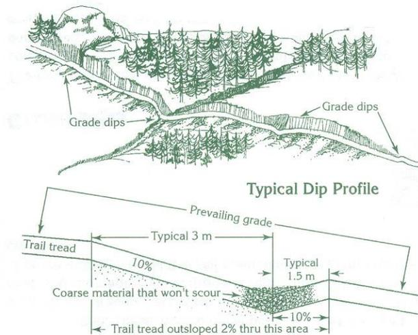
When you design and layout the trail, look for natural features to enhance the drainage. A rolling dip sometimes called terrain or grade dips are a great way to achieve this outcome. A rolling dip is simply a grade reversal to take advantage of a low spot to drain water off the trail.
