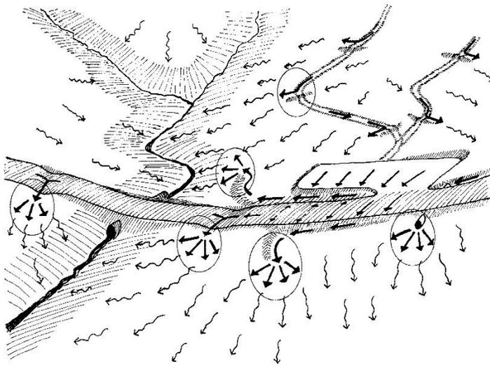
**BMPs typically minimize impacts to water quality by dispersing concentrated water flow. Circles indicate how BMPs disperse flow to the undisturbed ground.**
