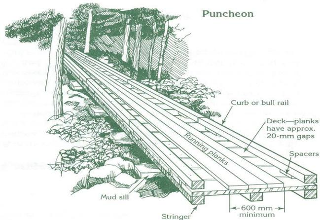
Puncheon is a wooden walkway (boardwalk) used to cross bogs or small streams. It consists of decking placed on stringers to elevate the trail across wet areas. It can be used and is preferred where rocky uneven terrain, muddy surfaces, or lack of mineral soils makes turnpike construction impractical. This is not generally suited for snowmobiles in areas that use wide and heavy trail groomers.
