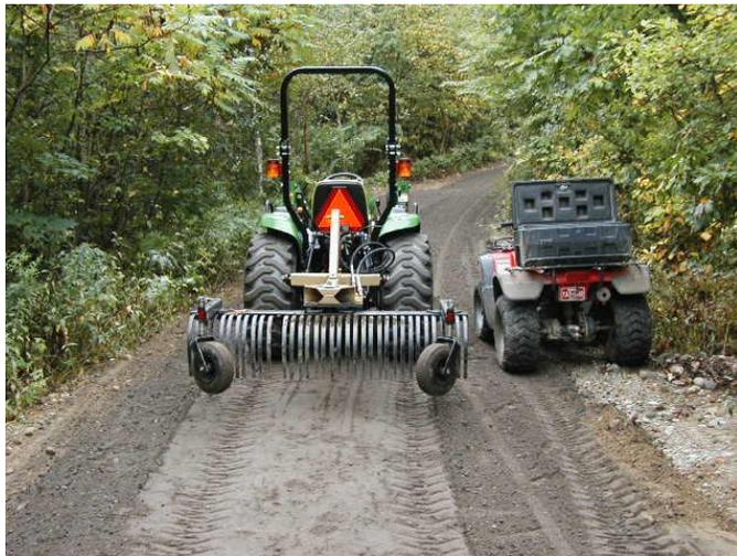
**A Steel tine rake, commonly called a York rake** is another affordable and effective piece of maintenance equipment. This device consists of a row of strong metal tines that work in much the same manner as a grader blade. They can be towed behind or mounted on the front of an ATV, tractor, or truck.
