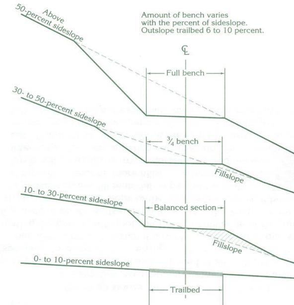
Steeper slopes may require a bench construction technique. Balanced bench construction uses some of the excavated soil for the trail. Be sure to remove all organic matter before you begin to compact your fill or the tread will settle and slump. While less stable than a full bench, a balanced bench takes less time to construct.
