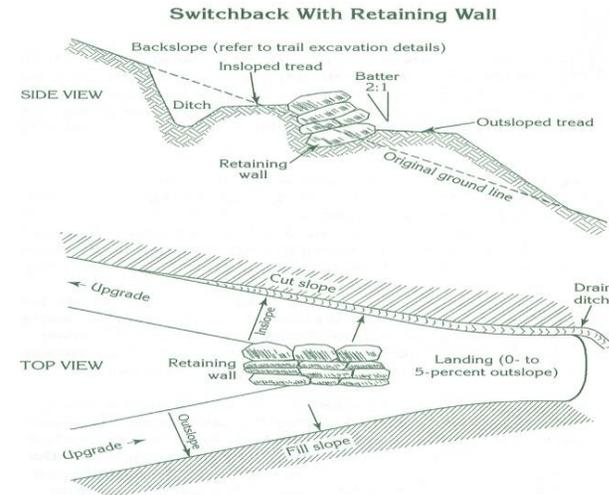
A switchback consists of upper and lower approaches, and a landing or turn platform. When scouting for switchback locations look for "natural" platforms. This will save you time later by reducing the amount of excavation needed.
