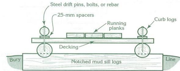
Stringers made from peeled logs or treated timbers are set on top of the mud sills. Stringers need to be level with each other so the surface will be level when the decking is added. Two stringers are usually enough for ATVs and snowmobiles, but for horses, three or four are recommended.
